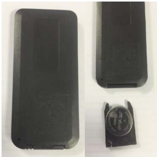
PUSH TAB TO THE RIGHT TO ALLOW BATTERY CASING TO BE REMOVED.
